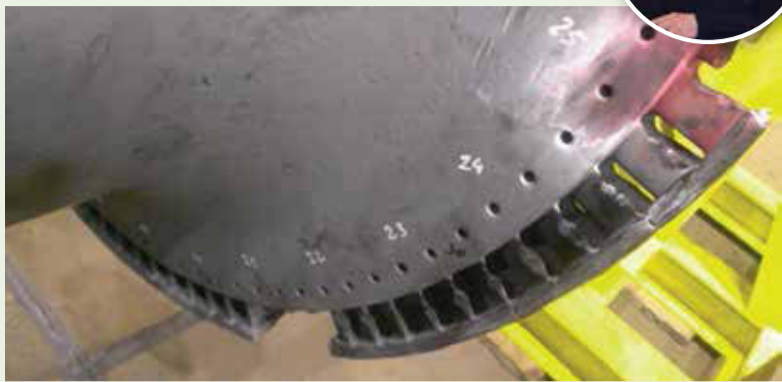
Photo shows the four missing blades on the first row of the rotating blades.
