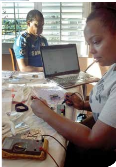
Above Conducting electrical testing of tricorder sensors
